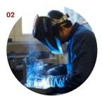
Folding and welding Workers fold and weld the pieces together to create the machine's shell.
